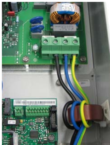
Figure 15: AC leads wound around the ferrite cores
