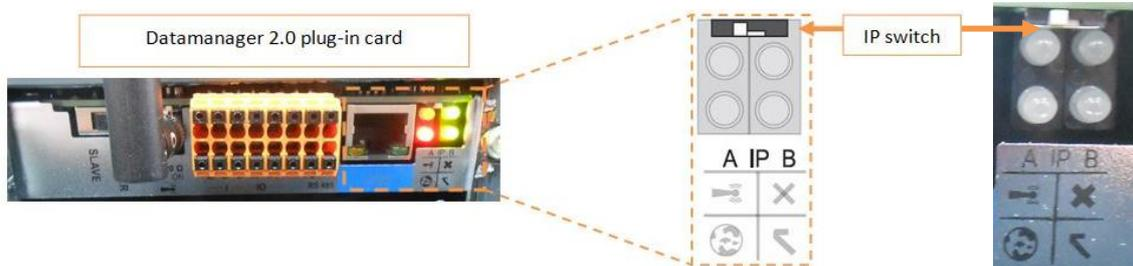
**Note:** Make sure to set the IP switch back to position B when the "Modbus Communication & Fall-Back Function Setting" section is complete otherwise the Fronius SCERT will not communicate to the SP PRO.
