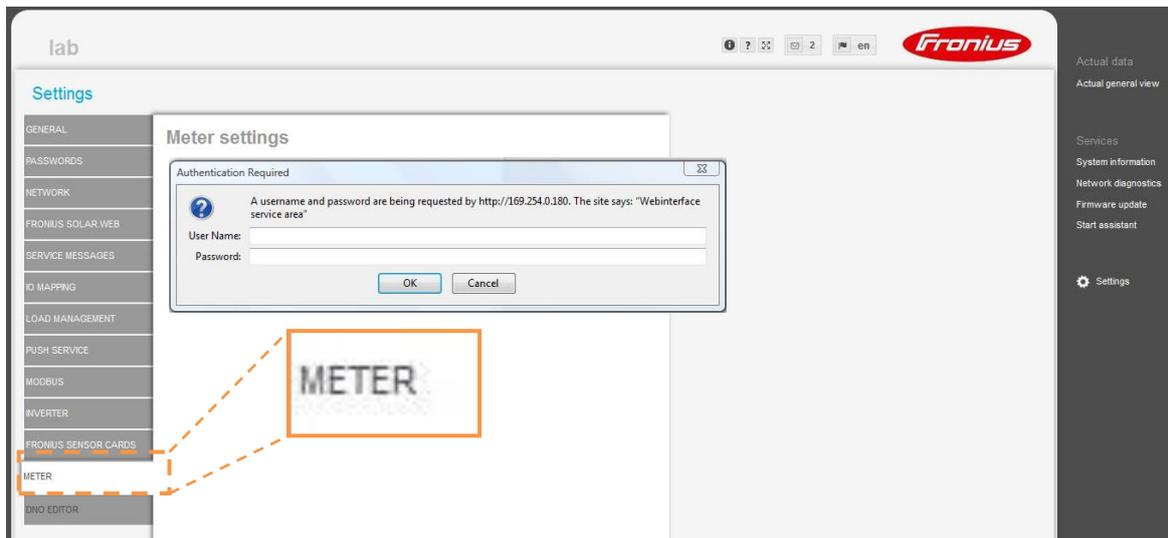
A user name and password are required to access the "METER" tab. Enter the service username and password created and then select "OK".
