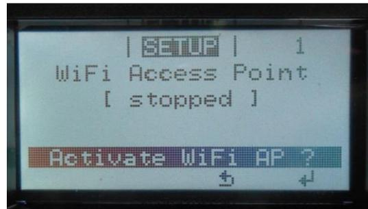
2. The "WiFi Access Point" will activate automatically "active" and the Network Name "SS" and Password "PW" will be displayed on the screen.
