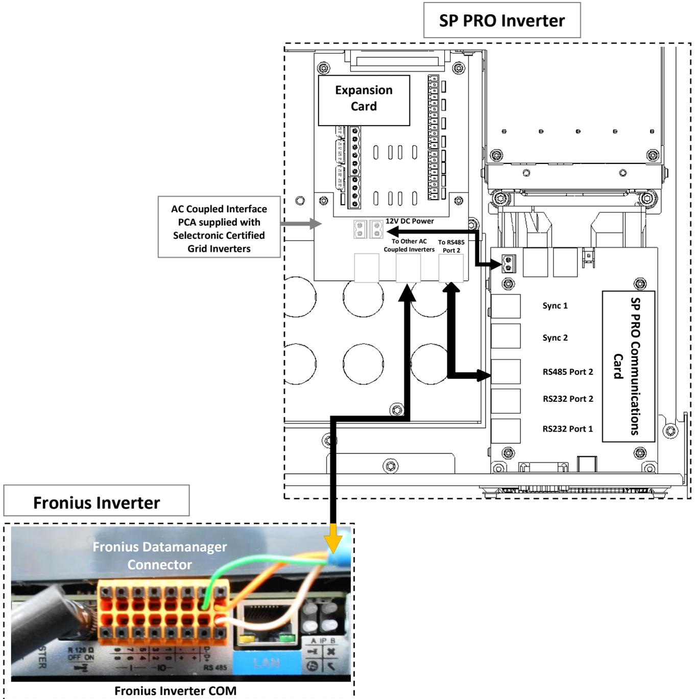
*SP PRO Connections (inside unit) – RS485 Port 2 RJ45 connector to AC Coupled Interface PCA and to Fronius Datamanager connector .*
