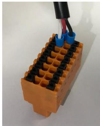
*Fronius SCERT Connections (inside unit) – RS485 Adapter Wires terminated into the Fronius Datamanager Connector.*
