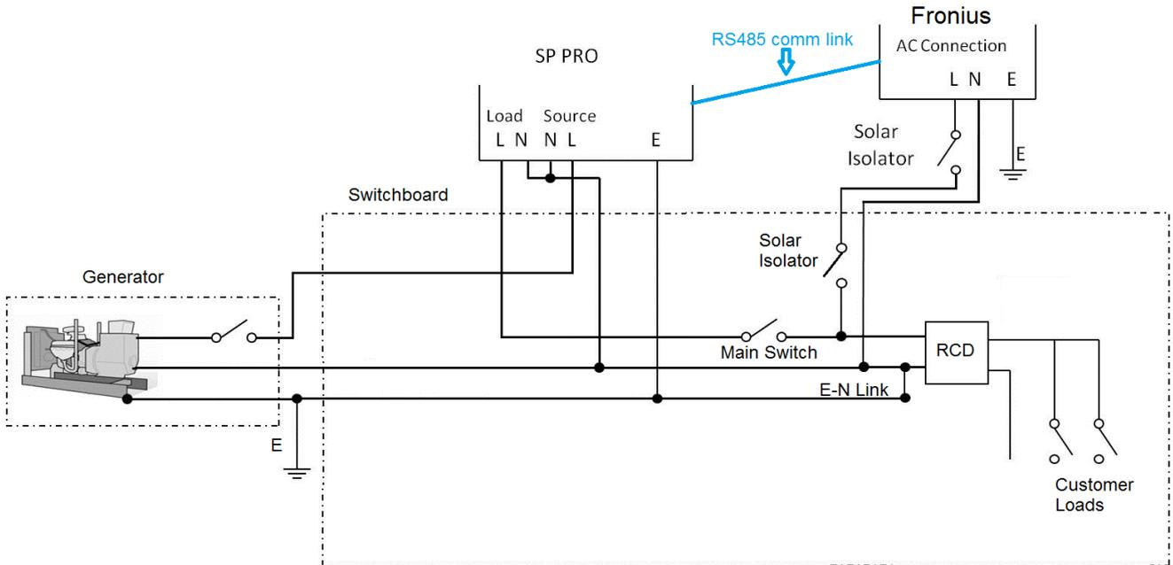
*Fronius AC Wiring guide for Off Grid installation*
