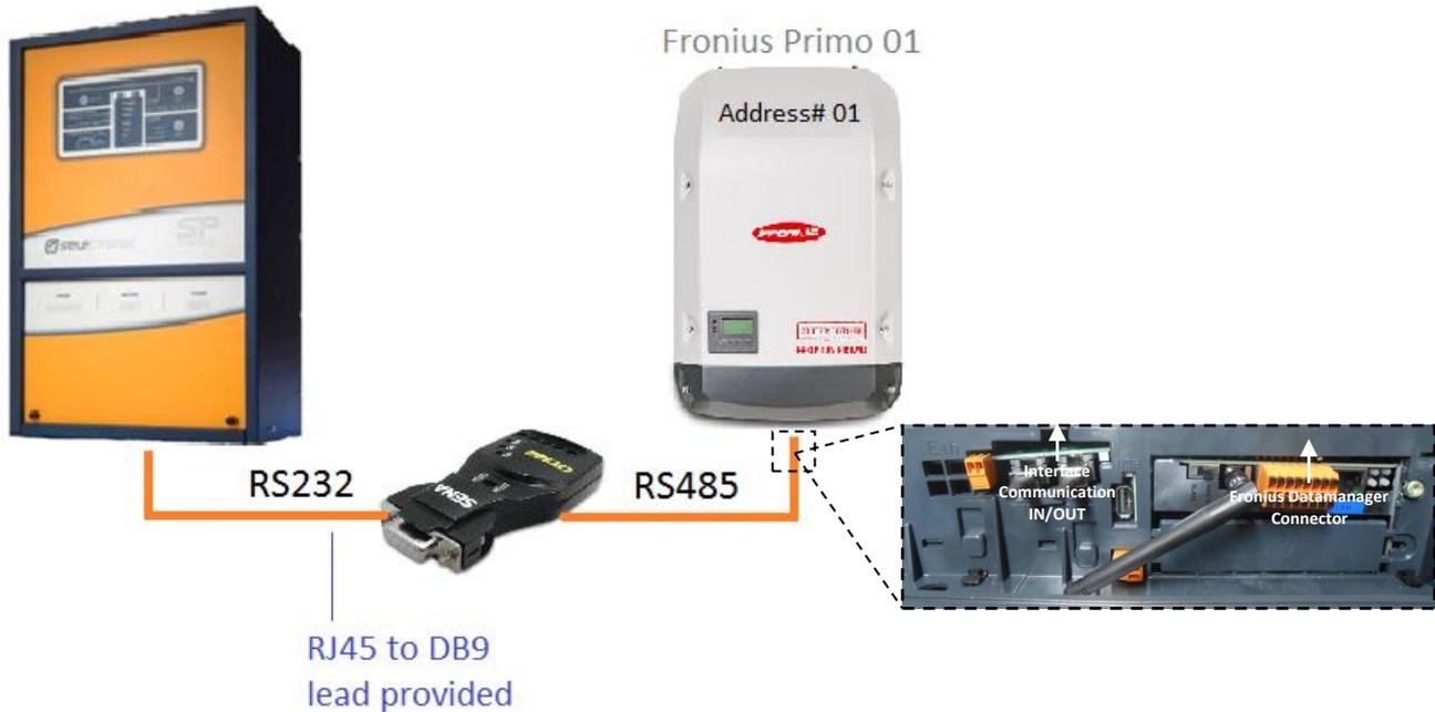
To install the Coupling adapter, use the RJ45 to DB9 lead and connect the Coupling adapter to the SP PRO Series I **Serial Port 2**. Then using 'CAT5' network cable or similar make, connect the Coupling adaptor to Fronius Primo 01 (Master) as per Table 1, Fronius Datamanager connector.
