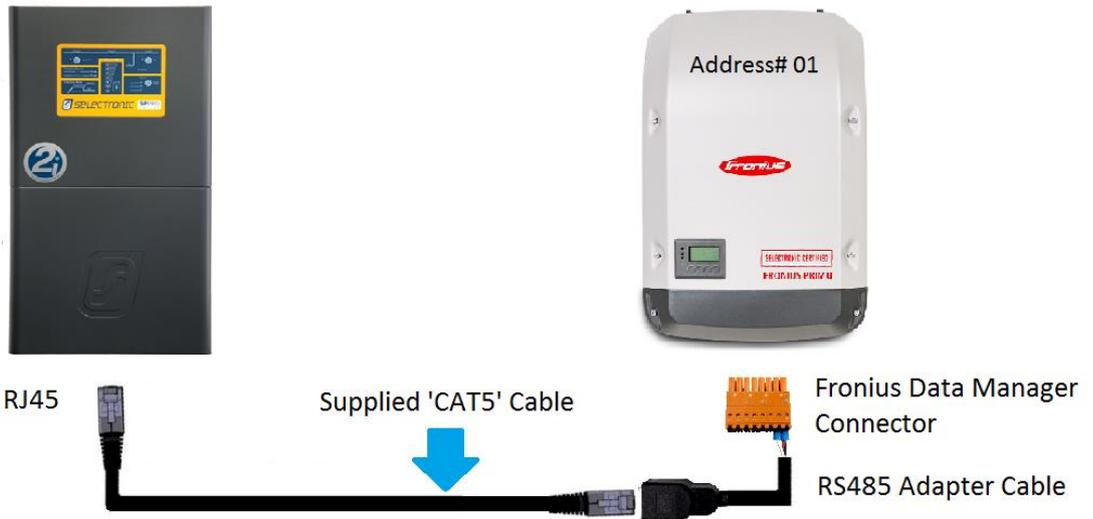
**The Fronius link connects subsequent Fronius SCERTs on the same SP PRO. Do not link together Fronius SCERTs that are on different SP PROs.**
