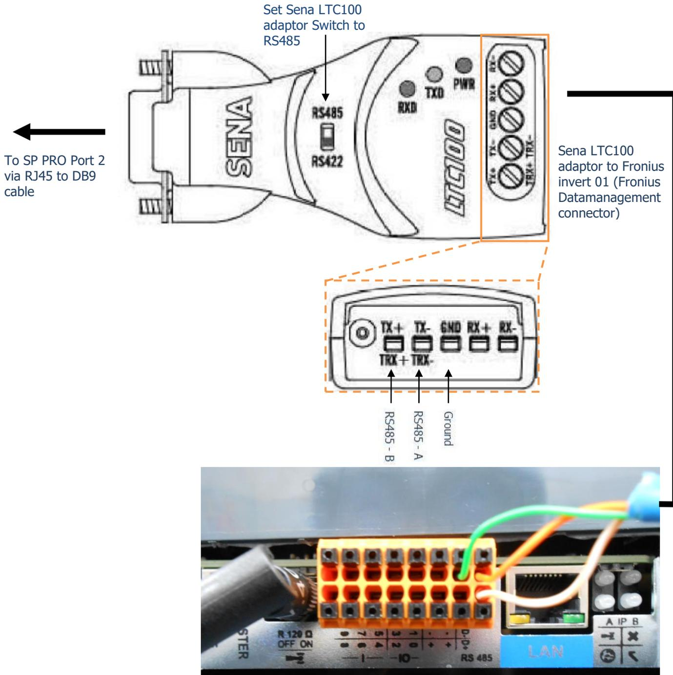
*SP PRO Port 2 RJ45 connector to Sena LTC100 and to Fronius Datamanager connector*
