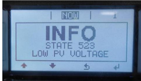
4. Once the display is active on the Fronius SCERT, access the main menu. To enter the main menu, press the **ESC** (↵) key once, then using the **LEFT** (←) or **RIGHT** (→) keys to scroll through the main menu. To access any of the menu items, press the **ENTER** (↵) key on the selected item. The **ESC** (↵) key is also used to return back to the previous menu or to edit previous digits.
