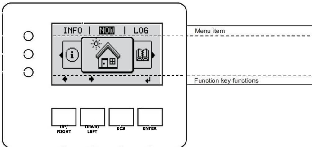
To access the **SETUP** menu, scroll once to the left and press the **ENTER** (↵) key. The **ENTER** (↵) key is used to confirm an action or to access submenus.
