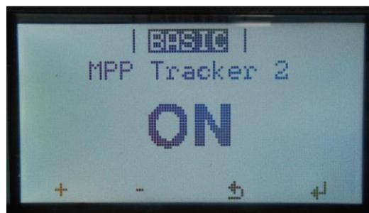
**Note:** When the Fronius SCERT is powered without the DC and the "MPP Tracker 2" is "ON", "INFO STATE 523 LOW PV VOLTAGE" will be displayed on the screen.
