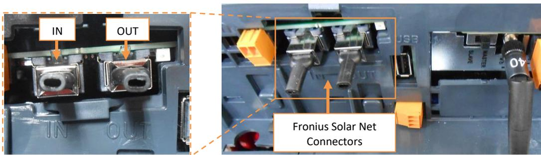
*Fronius Solar Net Connectors with termination: "IN" located on LHS & "OUT" located on RHS*
