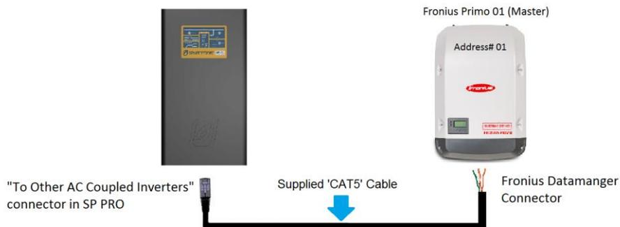
**The Fronius link is used to connect subsequent Fronius Primos on the same phase as the SP PRO. Do not connect Fronius Primos on different phases together.**
